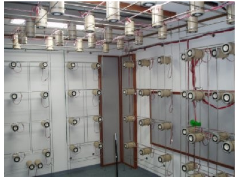
Surrounding speaker array (157 ch) FOSTEX FE38E (157 ch)
