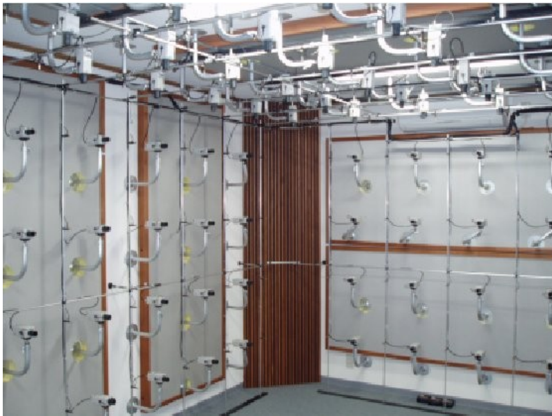
Surrounding microphone array (157 ch) B&K Type 4591 (157 ch)
