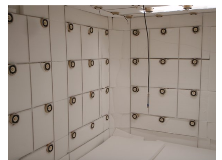
System latency measurement process using TSP signal
