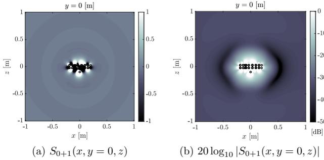
Figure 3: Results of conventional method using monopole pairs for  $f = 500$  Hz: (a) residual sound field  $S_{0+1}(x, y = 0, z)$  produced by  $D_0$  and  $D^{\text{even}+\text{odd}}$ ; (b) sound pressure level of residual sound field  $20 \log_{10} |S_{0+1}(x, y = 0, z)|$ .
