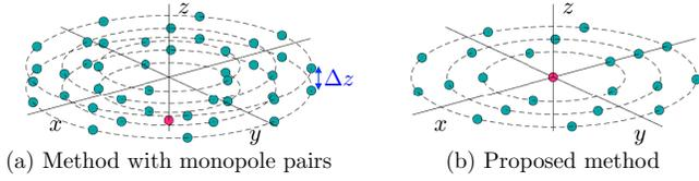
Figure 2: Arrangements of loudspeakers with three radii  $r_{1,2,3} = 0.1, 0.15$  and  $0.2$  m, where these circular arrays contain five, seven and nine loudspeakers, respectively: (a) conventional method using monopole pairs ( $\Delta z = 0.05$  m) with 43 loudspeakers, where the loudspeaker for  $D_0$  is located at  $[0, 0, -0.1]^T$  in Cartesian coordinates; (b) proposed method with planar array of 22 loudspeakers.
