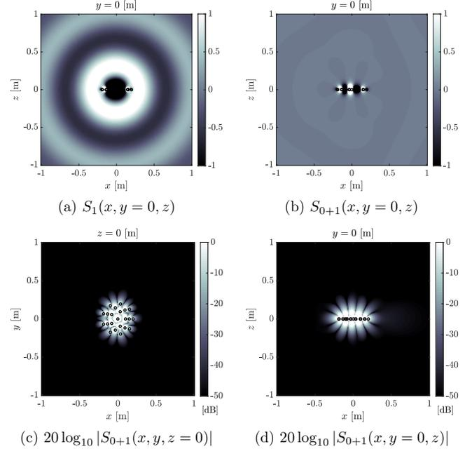
Figure 4: Results of proposed method for  $f = 500$  Hz: (a) sound field  $S_1(x, y = 0, z)$  produced by  $D$  using 21 loudspeakers; (b) residual sound field  $S_{0+1}(x, y = 0, z)$  produced using  $D_0$  and  $D$ ; (c), (d) sound pressure levels for the residual sound fields  $20 \log_{10} |S_{0+1}(x, y, z = 0)|$  and  $20 \log_{10} |S_{0+1}(x, y = 0, z)|$ , respectively.
